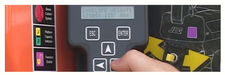
When it becomes necessary to replace a ground or power module on a JLG machine, it must be properly configured after installation. Use your JLG® Analyzer, or the new JLG® Mobile Analyzer, for configuration by accessing the "Machine Setup" menu and choosing the correct model and options appropriate to your machine.
